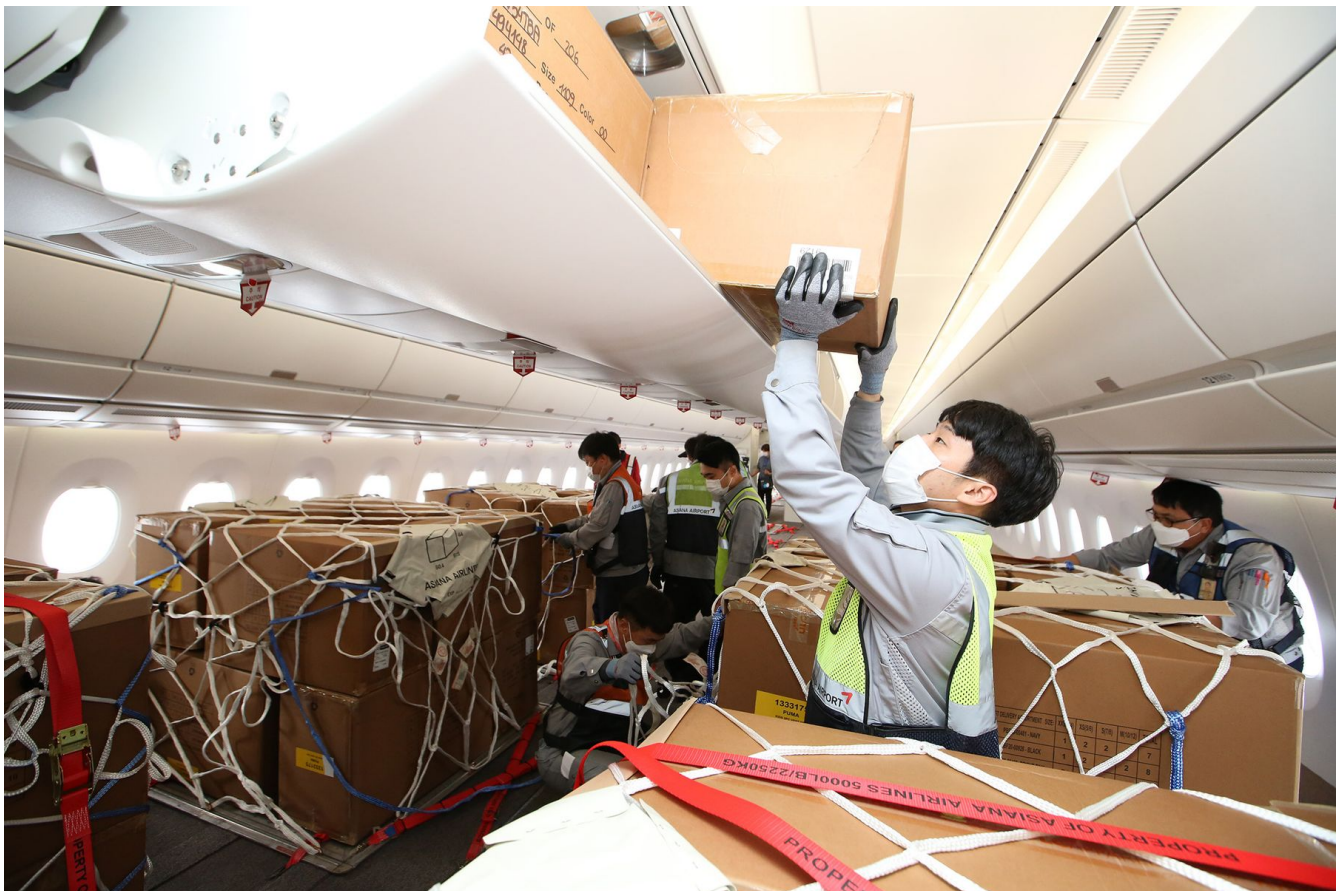
▲ Loading cargo on a converted Asiana Airlines Airbus A350. SOURCE: AIRBUS
